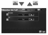
Selects a screen mode of the rear view camera (R-CAM) screen.
